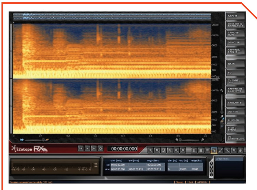
Figure 1: The stand-alone version of iZotope RX 2 Advanced. The right side of the GUI provides access to processing modules. Clicks in the audio file are displayed as three vertical lines in the center of the golden spectrogram, in which the floating waveform overlay is disabled.
